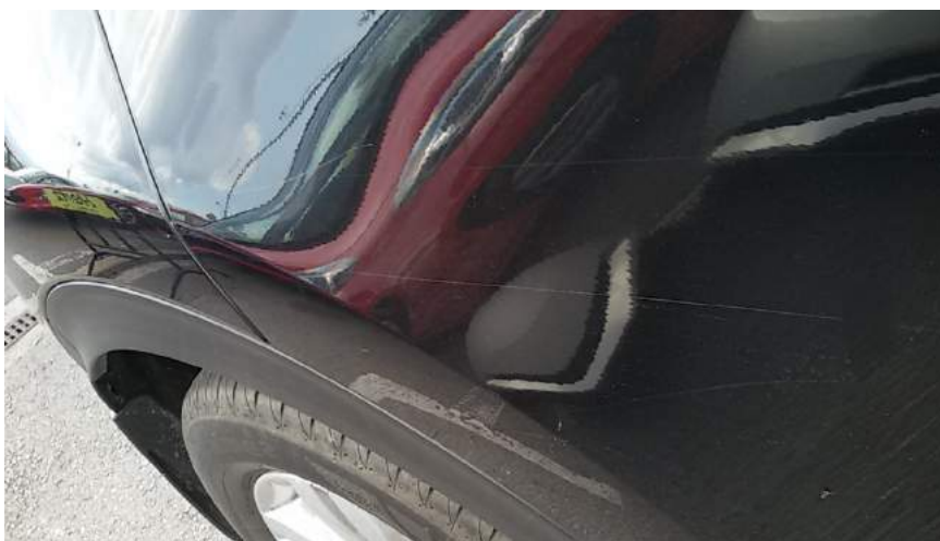
Scratches of the paint of the motor vehicle, which can be removed by polishing
